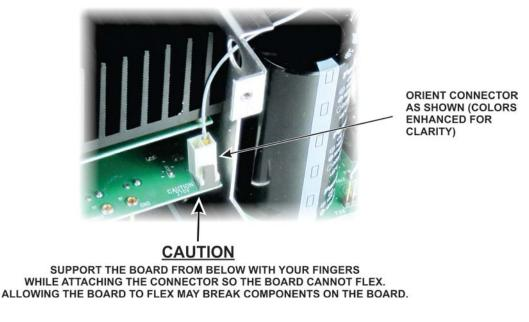
Figure 34. Connecting the 270V Wire to the PA/LPF Module.
